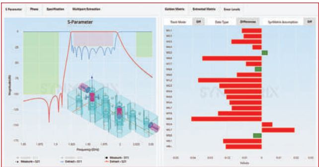
▲ Fig. 2 Computer-aided tuning with error indicators.
