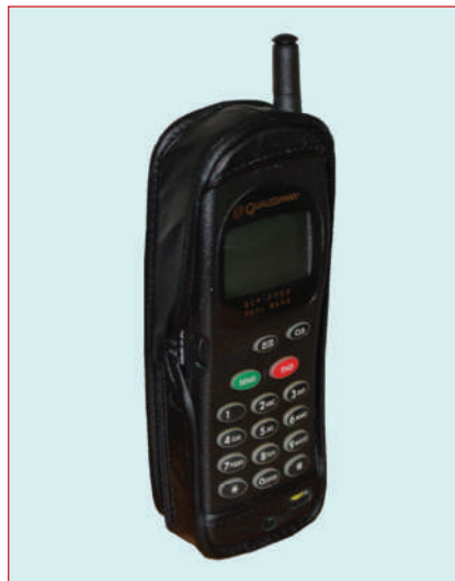
▲ Fig. 3 Qualcomm QCP-2700 cellular phone, which operated on the 800 MHz analog and 1900 MHz CDMA networks. Source: Ben Schumin, Wikimedia Commons.
